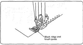
NOTE: These wires keep light weight tabric from rolling into a ridge and hold medium weight tabric flat.
